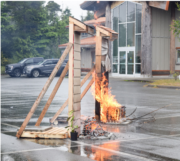
This photo shows the difference between the two house models after 20 minutes. While the fire on the left side has died out, the fire on the right side has spread to the structure.
